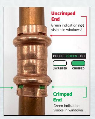
\* Green indication may show through windows prior to crimping. Once crimped, the green indication will expand, confirming a successful crimp.
